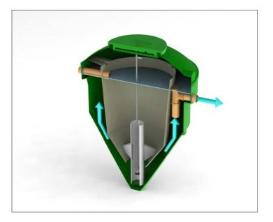
3: The treated liquid then exits through the dip pipe and is discharged safely in to the environment, meeting the required consent standard.
